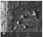
In direct comparison the picture on the right shows the same type spark plug after only 8 operating hours. As can clearly be seen molten surface material has already started to form beads on the surface and degrade spark plug performance.
