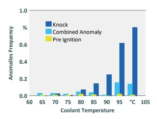
The picture shows a typical result of this method. As the coolant temperature increases, the frequency of anomalies rises significantly. Here, we can see that knocking is the main issue. These data are also available for individual cylinders.
